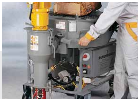
The material container and mixing tube are separated from each other. You open the gate valve and the material enters the mixing tube.
