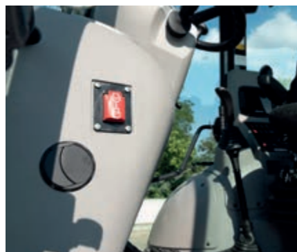
Secondary engine shut down switch
