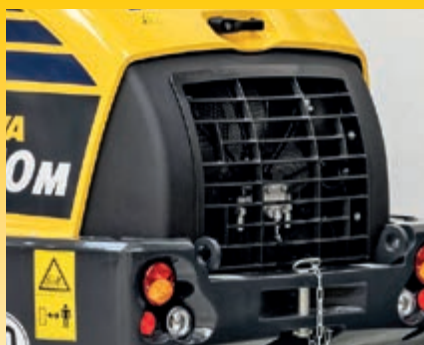
Wide core radiator with (optional) reversible fan
