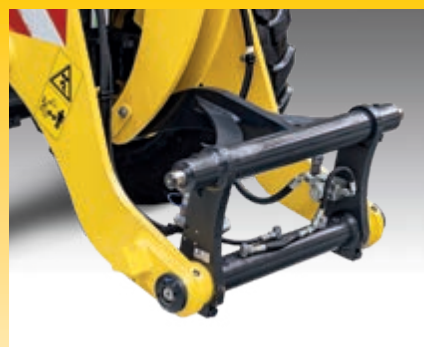
Electrically actuated quick-coupler for fast and easy change of attachments
