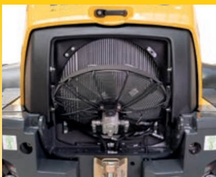
Tiltable radiator fan for convenient cleaning access
